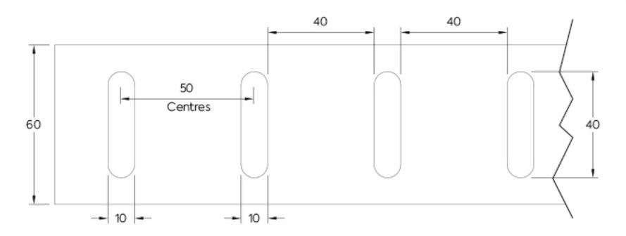
The Dentil rail is supplied at 2540mm long x 60mm high – groove positions are as shown, at 50mm spacings, giving 40mm gaps between grooves. Please consider this when cutting the Dentil rail, to ensure grooves are centrally positioned across the cut length.
