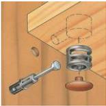
The head of the metal dowel will fit into the cam and once in place the cam is screwed tight to secure the panels.
