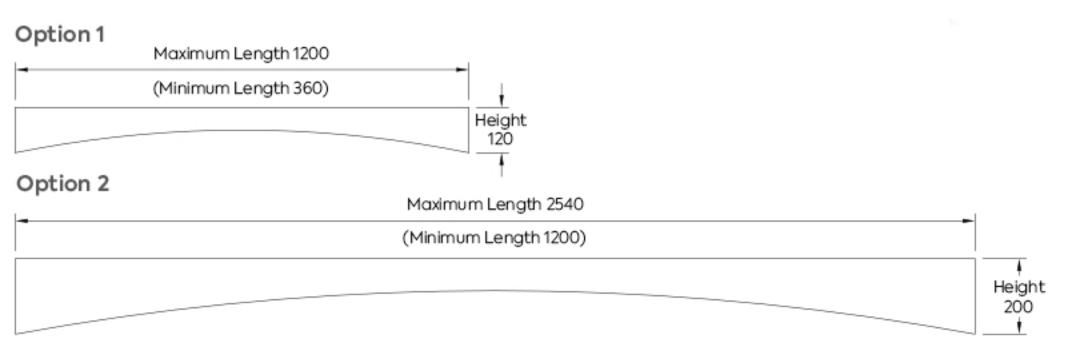
The Arched pelmet is offered in two heights – 120mm high for lengths supplied from 360 mm to 1200mm – and 200mm high for lengths supplied 1200mm to 2540mm. They can be used for a variety of applications, such as window pelmets (as shown below) or also in bedroom applications, to create design features over beds.
