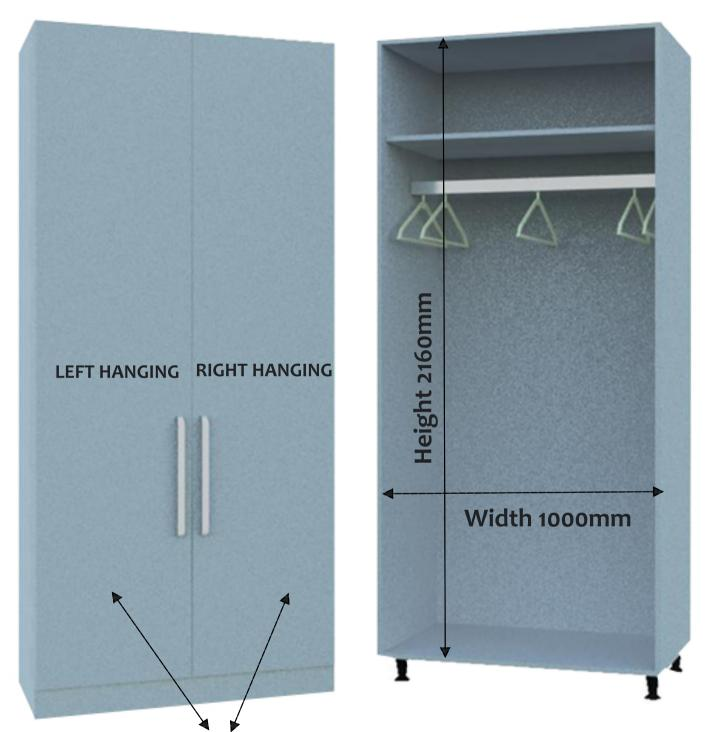
To establish if a door is left or right hanging for hinge holes view the door from the front
